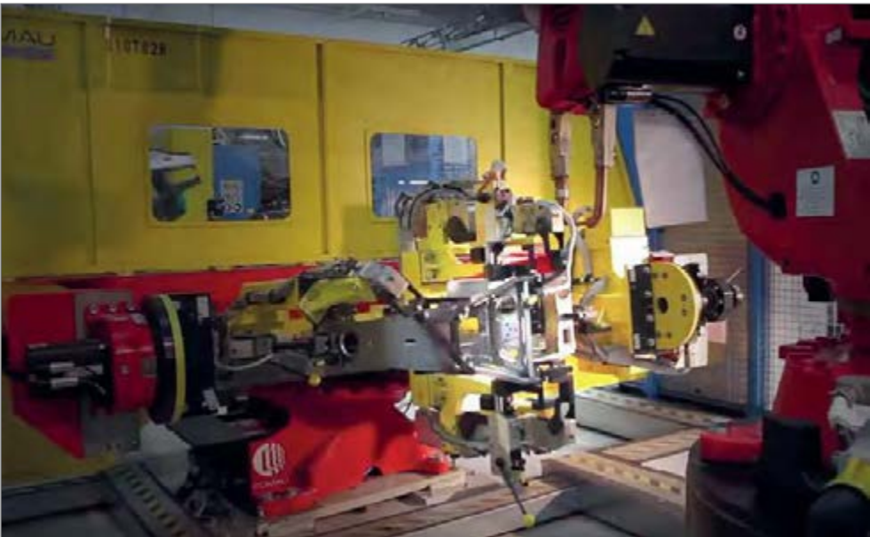
Fig. 7.23. Welding of the components of the Vespa Primavera scooter at Piaggio (source: COMAU Robotics)
