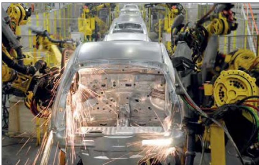
Fig. 7.21. FANUC robot during car body welding (source: www.robotco.com )
