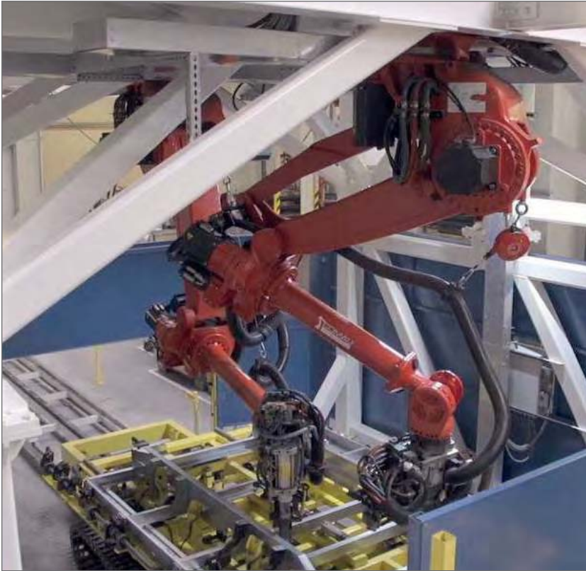
Fig. 7.22. Spot welding of transport trailers in Kostrzyn (source: COMAU Robotics)
